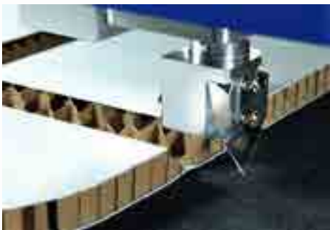
XVT - V cutting tool, perfect for POS and displays using hexacomb board.
