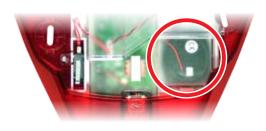
**Engineer hold-off facility.** The Deltabell E's engineer hold-off facility means that when initially powered with the tamper switch open, the sounder will not activate.
