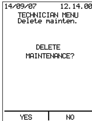
Press YES to delete all maintenance interventions performed on the steriliser from the machine memory and reset the remaining day and cycle counters for all components. Press NO to keep the maintenance log and go back to the Technician Menu.
