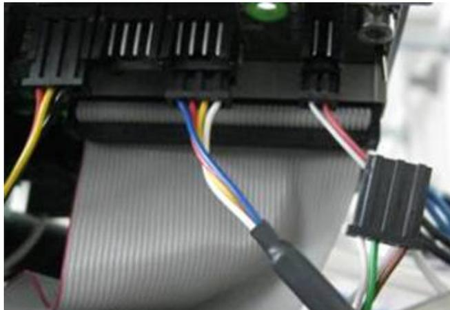
Connect the 4 pin cable of the calibration tool to connector CN11 of the power board.
