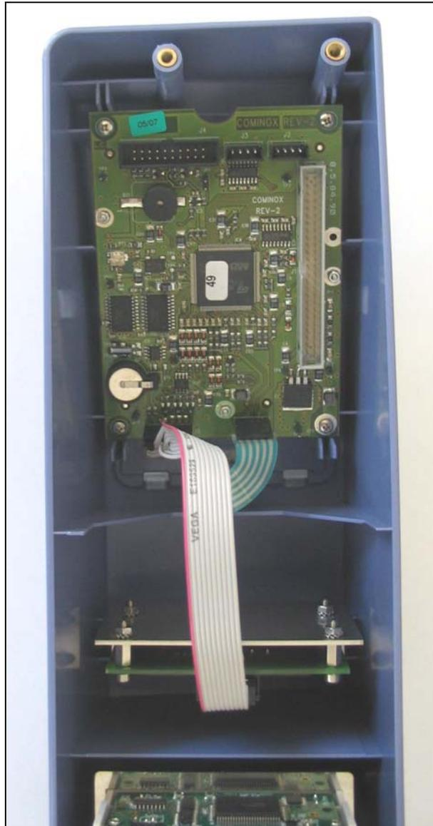
**Note:** The assembly must be placed as high as possible, so that the opening of the control panel is aligned with the one of the SterilCard reader.
