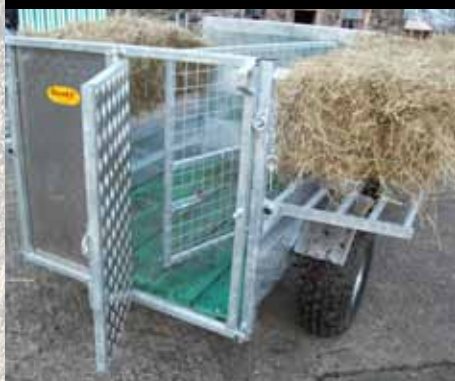
5x3'3 folding sided trailer with lamb partition and ramp door with integral swing model shown
