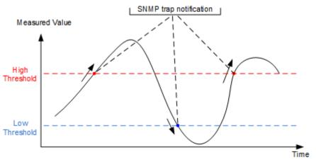
Figure 7.20. Sending traps with Traps Sending=Level Triggered
