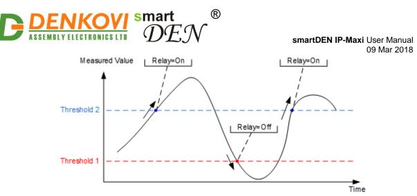
Figure 7.24. Inverse mode: AI Threshold 1 < AI Threshold 2
