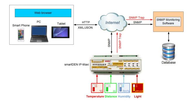
Figure 2.2. Remote sensors monitoring
