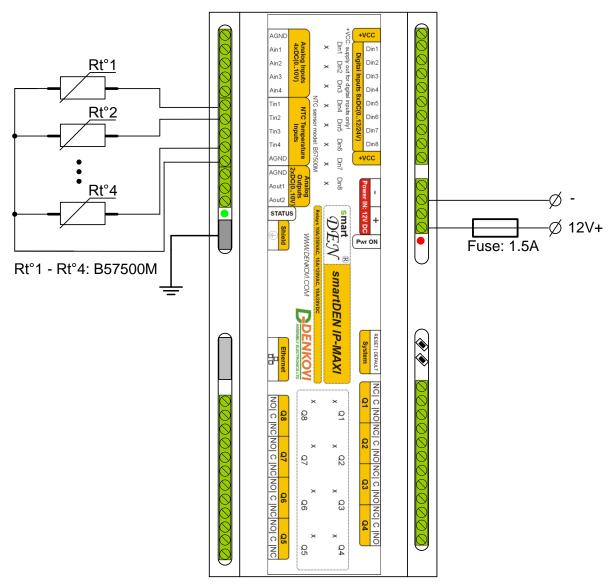
Figure 5.7. Connecting NTC sensors type B57500M to the Temperature Inputs
