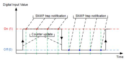
Figure 7.18. SNMP Trap Value="2 (Both)", Trap Sending="Level Triggered"
