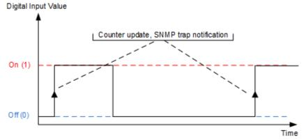
Figure 7.15. SNMP Trap Value="1 (On)", Trap Sending="Edge Triggered"
