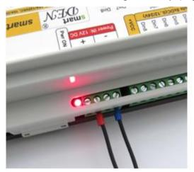
Figure 5.2. smartDEN IP-Maxi power supply
