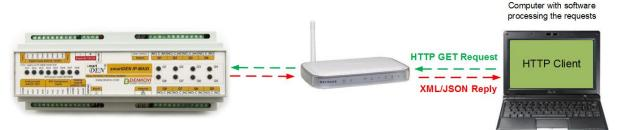
Figure 8.1. smartDEN IP-Maxi working as a HTTP server
