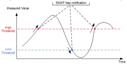
Figure 7.21. Sending traps with Traps Sending=Edge Triggered
