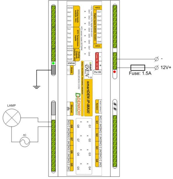
Figure 5.8. Connecting lamp to relay
