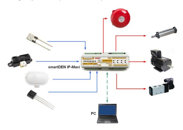
Figure 2.3. Standalone control of electrical devices
