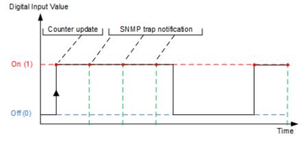
Figure 7.16. SNMP Trap Value="1 (On)", Trap Sending="Level Triggered"
