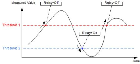
Figure 7.23. Normal mode: AI Threshold 1 > AI Threshold 2
