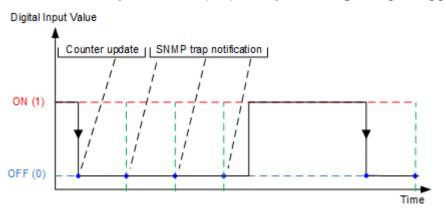
Figure 7.14. SNMP Trap Value="0 (Off)", Trap Sending="Level Triggered"
