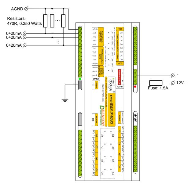
Figure 5.5. Connecting 0-20 mA output sensors to the Analog Inputs
