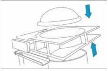
A top tube assembly goes through the roofing materials
