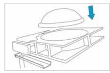
A dome sits on the roof flashing
