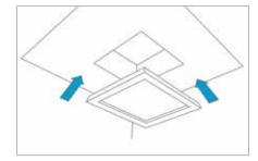
A diffuser which is fixed flush to the ceiling
