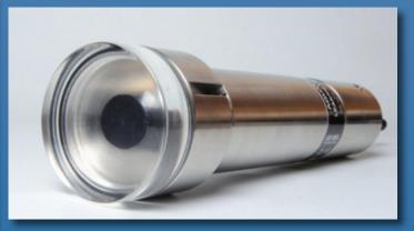
The sensors have a single forward facing light source (like a torch) producing a 'tuned' high intensity beam of excitation light that spreads to about 45cm diameter at 3m from source (and continues spreading as the distance increases). Fluoresced light is generated when the beam encounteres leaked fluid. This fluoresced light is detected by a sensor mounted concentrically round the light source.
