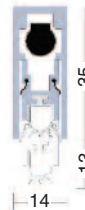
LAS 801si Available in widths from 335mm to 1235mm, can be cut back 99mm (Except 335mm which cuts back to 80mm).
