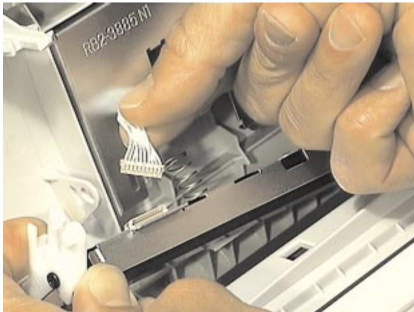
Figure 4-6 Disconnecting the CIS wire connector
