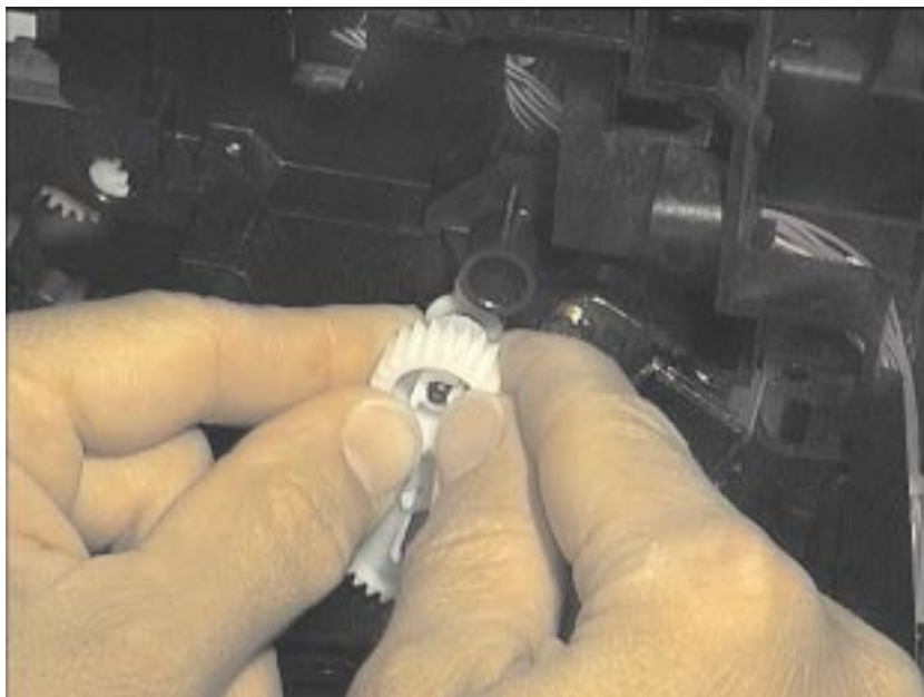
Figure 4-52 Removing the paper feed assembly (continued)
