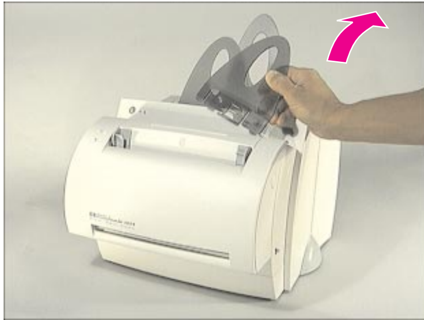
Figure 4-1 Removing the paper guides
