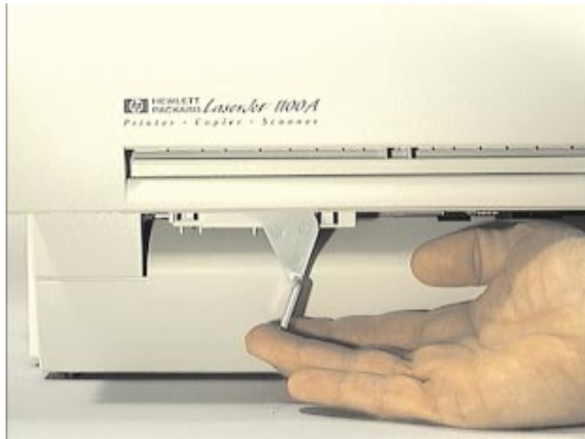
Figure 4-2 Removing the optional scanner unit
