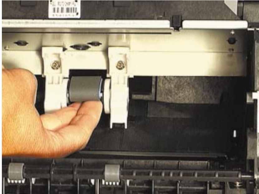
Figure 4-38 Changing the pickup roller
