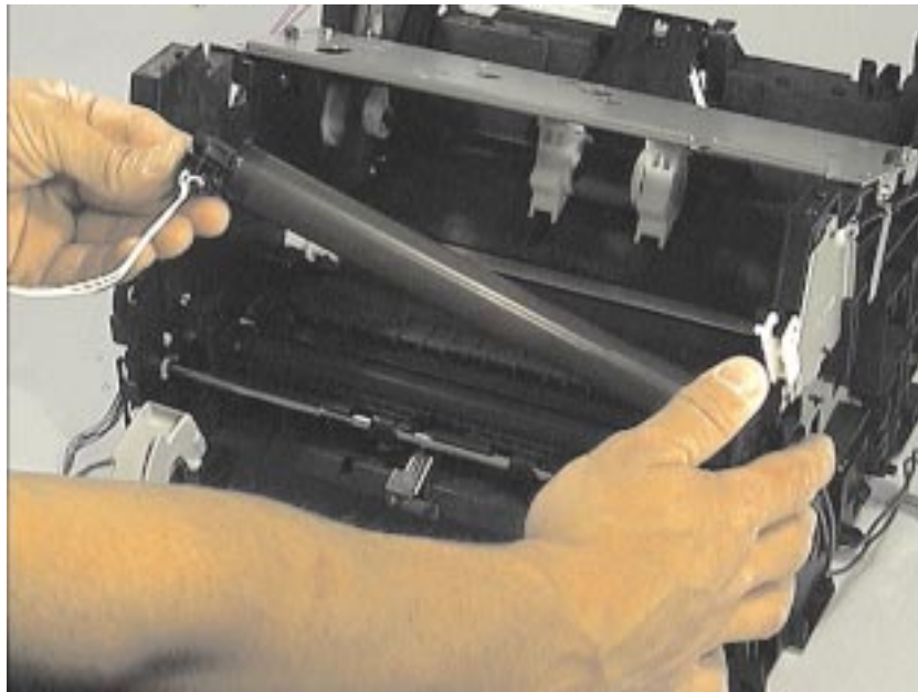
Figure 4-31 Removing the fusing element
