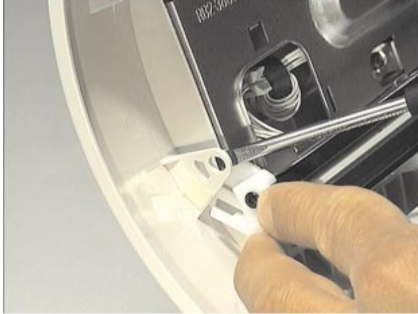
Figure 4-5 Removing the Contact Image Sensor (continued)
