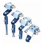
The B Manifolds are specialized transition blocks with multiple spray points set at ideal angles to lubricate the teeth, gullet, and sides of a circular saw blade. B Manifolds incorporate Wet Tips to generate a high velocity spray that can penetrate the wind force typical of high speed sawing for maximum tool life with minimal
