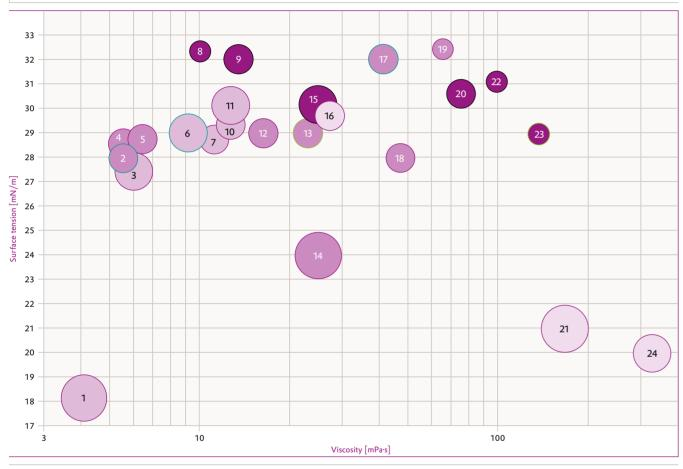
Size of circles: proportional to spreadability. The smaller/bigger the size of circle the lower/higher the spreadability. Color of circles: very high polar < > \boxtime non-polar.
