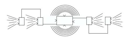
directions. In a general arable situation the slave units give valuable extra protection when directed towards peripheral trees/power lines where birds tend to perch before feeding. Slave units are available as end units with one socket, or intermediate units with two sockets.
