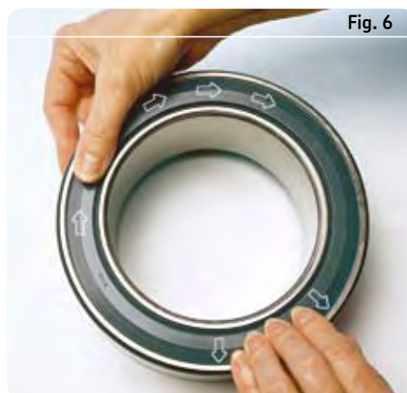
Inserting the seal in the outer ring
