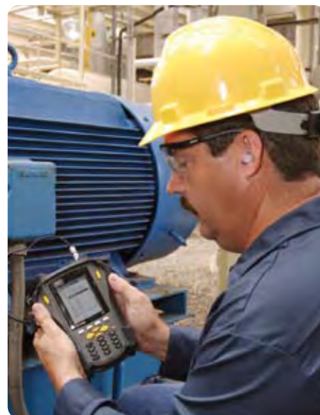
Recording vibration values using a SKF Microlog Series Data Collector
