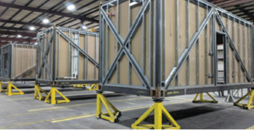
Modular units can be constructed indoors, limiting weather-related delays and improving quality control.
