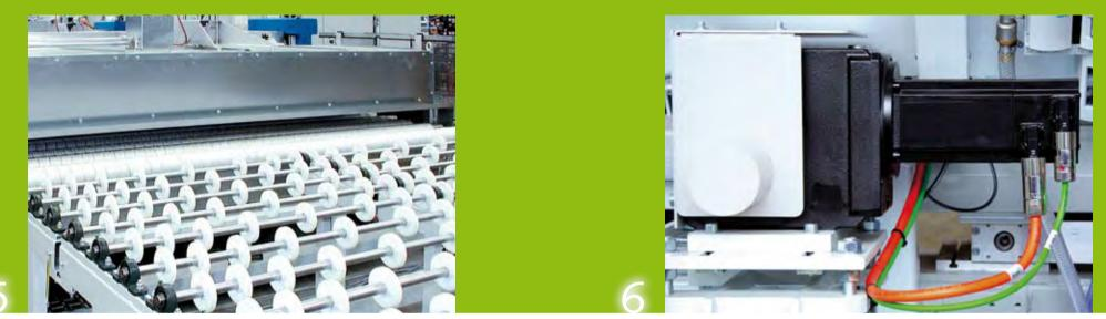
In photovoltaic module production, we replace the vacuum laminators by a pre-nip with press rollers.
