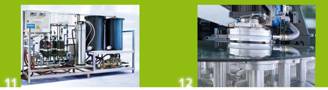
We have drastically reduced water consumption in insulating glass production. We can achieve this by using a closed water circuit with disc filter system. All in all, consumption is reduced by up to 15 times. During deceleration at the drives of the automotive glass plants, we convert kinetic energy into electrical energy and feed it back into the network. This produces energy savings of up to 20%.
