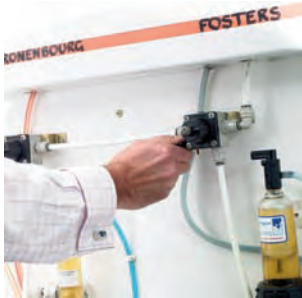
1. Switch off gas supply
