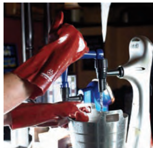
8. Allow cleaning solution to soak in the lines for 10 minutes, pull fresh solution through each line
