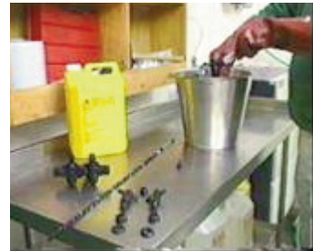
Clean cask taps and dipsticks
