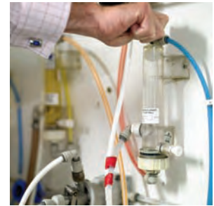
6. Refill the cellar buoy with cleaning solution
