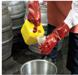
5. Following manufacturer's instructions, add cleaning fluid to the cleaning bottle
