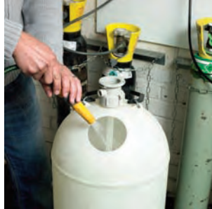
2. Fill the cleaning bottle with clean cold water and connect keg couplers to cleaning sockets
