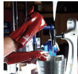
9. After a further 10 minutes, pull fresh solution through each line
