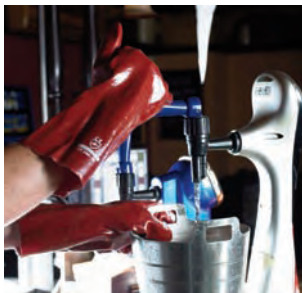
7. Pull cleaning solution through to each tap (avoid cleaning more than 4 taps at any one time)
