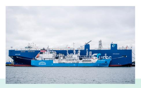
carriers (PCTCs) in 1H 2017. The ENGIE Zeebrugge loads LNG at Fluxys' LNG terminal in Zeebrugge, where small carriers with capacities from 2,000 cum upwards can dock at the second jetty which was commissioned in January 2017.
