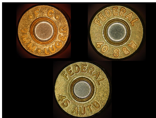
Figure 3: Samples of headstamps (upper). Small pistol primer on Federal .45 Auto cartridge (lower)
