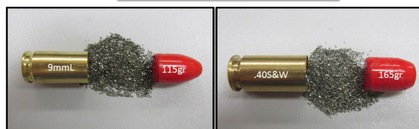
Figure 2: Intact and disassembled 9mm and .40 S&W cartridges
