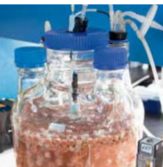
Above, top: Kartik Chandran (Photo by Tim Lee Photographers); bottom: A highly cost-effective and energy-efficient technology for biological nitrogen removal from wastewater using anaerobic ammonia oxidizing (anammox) bacteria that is being developed by Kartik Chandran's group (Photo by Jeffrey Schifman)
