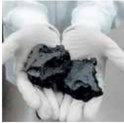
Above, top: Alissa Park (Photo by Eileen Barroso); bottom: Rethinking waste to complete material cycles for sustainability like the steel slags pictured here, an example of the unconventional resources containing rare earth elements.
