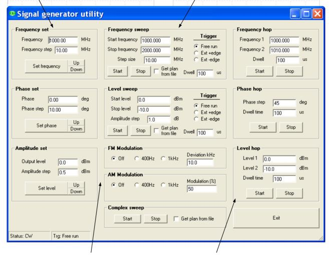
**FM and AM** modulation modes at 1 kHz or 400 Hz with up to 200 kHz FM deviation and up to 90% AM modulation depth.
