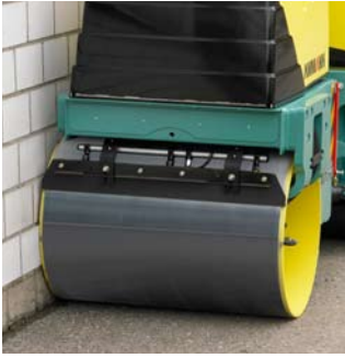
Compaction up against walls and boardways
