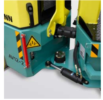
Life time lubricated teflon central articulation joint
