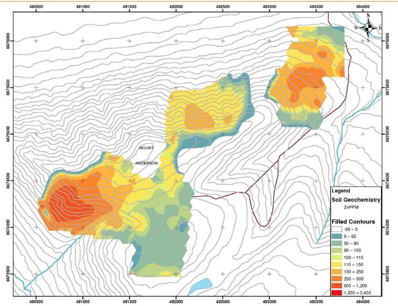
Figure 12: Zn in Soils, 2011 (Apex Resources Inc.)
