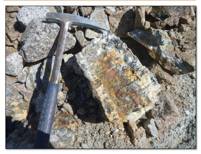
Figure 5: Banded quartz-galena veining, 47-Zone
