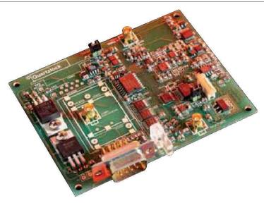
The A6-CPS digital phase locked loop (PLL) provides an low noise, very high short term stability filtered output which can be customised to a specific application.
