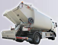
Lifting containers manufactured to British Standard EN840-1 or EN840-2 up to 660ltr, the binlift can also be easily configured to accept a bin weigh system ensuring all rounds maximise the available payload while remaining within legal limits. There is also the option of additional high level controls for the emptying of containers situated above ground level - useful for distribution centres and loading docks.
