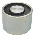
This magnet exerts a holding force of approximately 40 Kgf perpendicular to any steel plate (see accessories) with which it is in contact, assuming nominal voltage, and coil at working temperature rise of 60°C in an ambient of 20°C.
