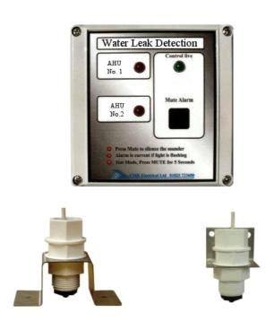
The unit has been designed to monitor critical areas for water leaks via remote optical sensors. Up to two sensors can be connected to a zone.
