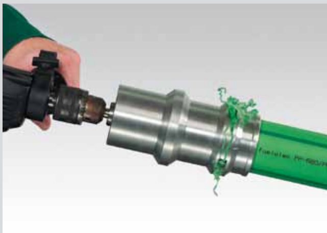
aquatherm peeling tool (Art.-No. 50558-70, up to 75 mm) (from 90-160 mm: Art.-No. 50572-50592 (without picture))
