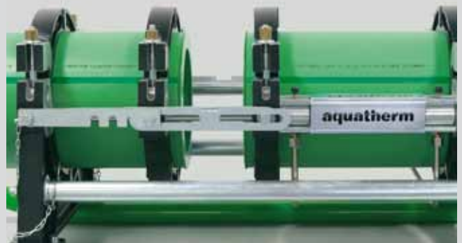
Divide the machine slide, remove heating element
