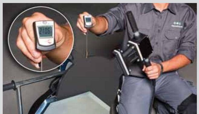
Measurement of temperature at the aquatherm butt-welding machine
