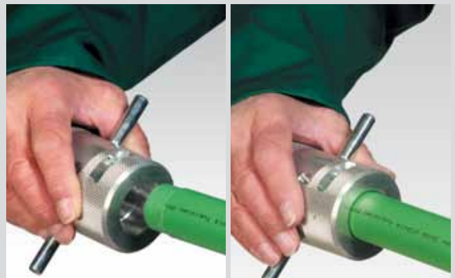
Peeling of the aluminium-PP-composite-layer respectively oxygen barrier layer (Necessary only for stabi-composite pipes and aquatherm blue pipe OT)
