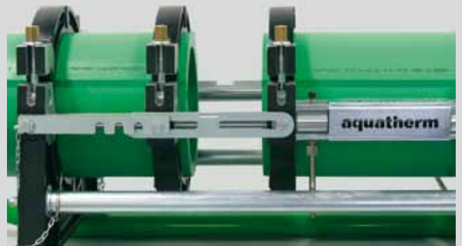
The parts to be welded are fixed and aligned respectively, the milling machine is used
