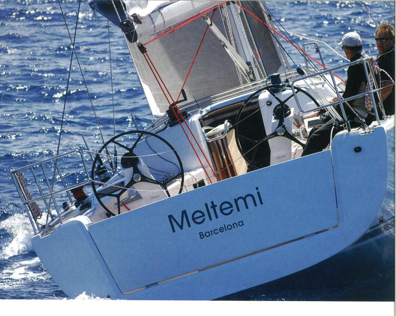
Race primaries are also well sited with a good working area for the racing crew but not too far forward for short handed sailing. The slanted coamings are great for the trimming team, even when the boat is very well heeled. The side decks and foredeck represent good working areas, our test boat was trimmed with the teak deck option.
