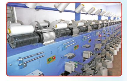
Assembly winder with individual length controller and cutter.
