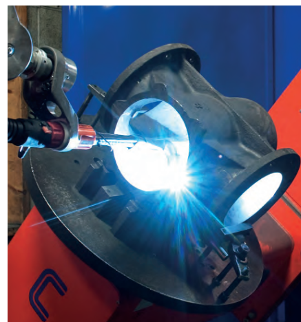
Figure 3. Robotic welding of nickel seat
