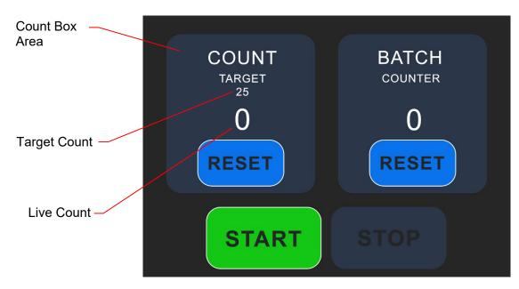
• The **COUNT SECTION** of the interface displays the predefined **TARGET COUNT**. As tablets are processed by the count sensor a live count is displayed in real time. This provides the operator with live data of the productions progress.
