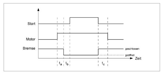
When switching on the controller, the brake becomes active first and the motor is not provided with power. First the motor current is switched on and a period of ta ms waited. Then the brake is disengaged and a period of tb ms waited. Travel commands will only be executed after expiration of ta and tb.
