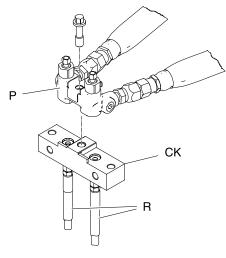
The Fusion AP gun manifold is shown.
