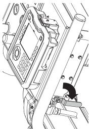
9. Turn main power switch OFF. Allow engine cooling dwell time prior to shutting down the engine.
