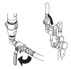
12. Engage gun piston safety lock then close fluid inlet valves A and B.
