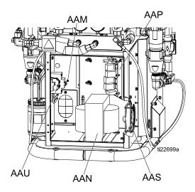
AAM Hose Breaker AAN Transformer AAP Load Center AAS Fan AAU Wiring Terminal Blocks
