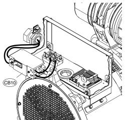
Figure 15 Circuit Breakers Inside Alternator Assembly
