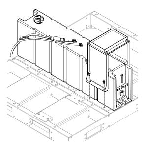
Remove Battery Bracket and Fuel Tank Figure 21
