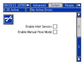
2. Manual hose mode is automatically disabled when the system detects a valid RTD sensor in the hose.
