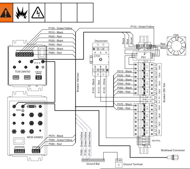
Figure 13 Circuit Breaker Connections Inside Electrical Enclosure (DB)
