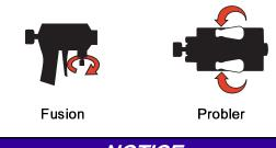
**NOTICE** To prevent crossover on impingement guns, **never** open fluid manifold valves or trigger gun if pressures are imbalanced.
