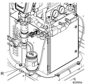
Figure 29 Component A Pump
