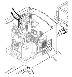
Radiator Exhaust and Air Intake Louvers Figure 20
