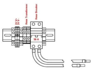
Figure 14 Circuit Breakers Inside Proportioner Cabinet
