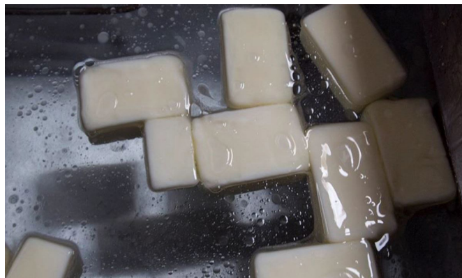
Lard melting in sink bowls before draining, at Mechline's testing facility.
