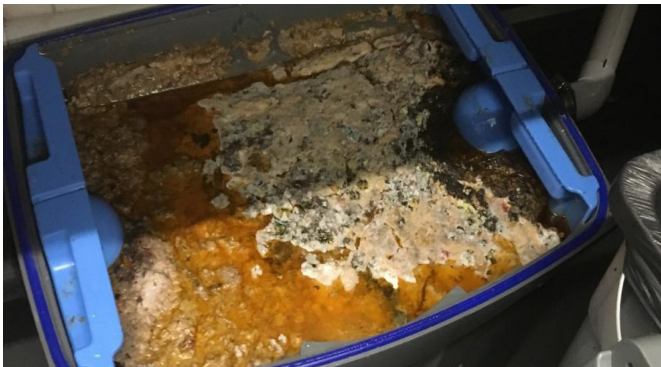
17 August 2017 - 20 days in. Floating organic around 150mm from surface.
