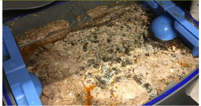
9 August 2017 - 12 days in. Floating organics around 100mm deep from surface.
