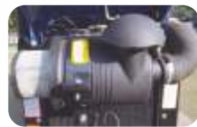
DRY TYPE AIR CLEANER WITH CLOGGING SENSOR
