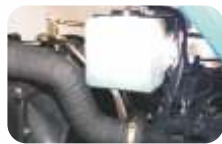
RADIATOR OVERFLOW RESERVIOR (No need to fill coolant again & again)
