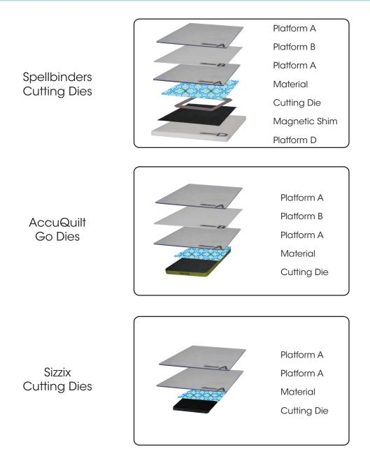
Important: When using AccuQuilt Go dies or Sizzix cutting dies, do not have fabric hang over the dies or risk jamming the machine.
