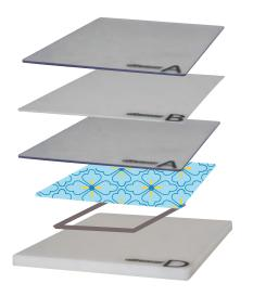
Platform A Platform B Platform A Material Cutting Die Platform D
