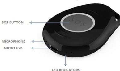
When the battery is running lower than 20%, it will send an SMS alarm 'BAT:LOW' to all preset numbers.
