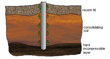
Piles that pass through layers of moderately- to poorly-compacted fill will be affected by **negative skin friction**, which produces a downward drag along the pile shaft and therefore an additional load on the pile. This occurs as the fill consolidates under its own weight.
