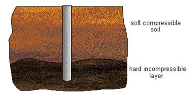
End bearing piles are those which terminate in hard, relatively impenetrable material such as rock or very dense sand and gravel. They derive most of their carrying capacity from the resistance of the stratum at the toe of the pile.
