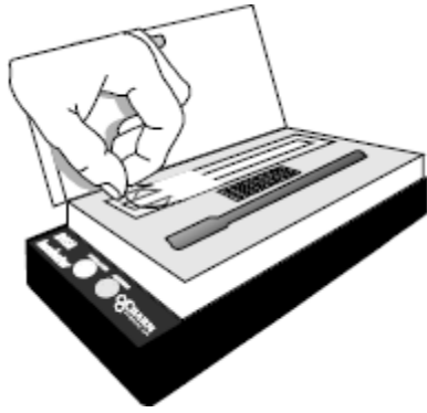
Figure 33: A graphical representation showing a test strip being placed in a Charm ® incubator (Charm Sciences Inc, 2009).
