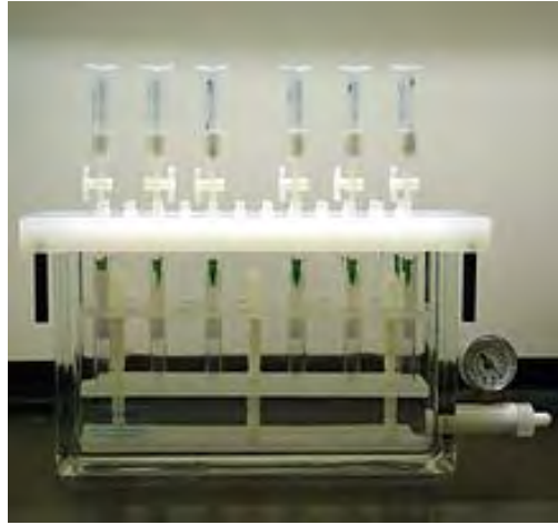
Figure 32: A photograph of a typical solid phase extraction manifold. The cartridges drip into the chamber below, where tubes collect the effluent. A vacuum port with gauge is then used to control the vacuum applied to the chamber (Wikipedia, 2011).
