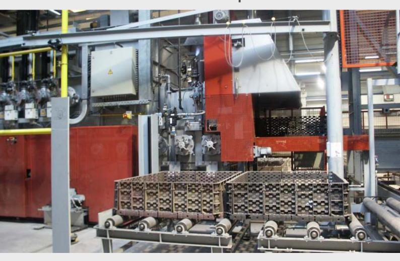
for heat treatment of forging parts under atmosphere
