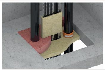
QF2 Fire Protection Compound used in conjunction with MW Mineral Wool Slab
