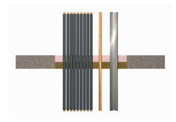
Cross section of QF2 Fire Protection Compound used in a floor in conjunction with MW Mineral Wool Slab
