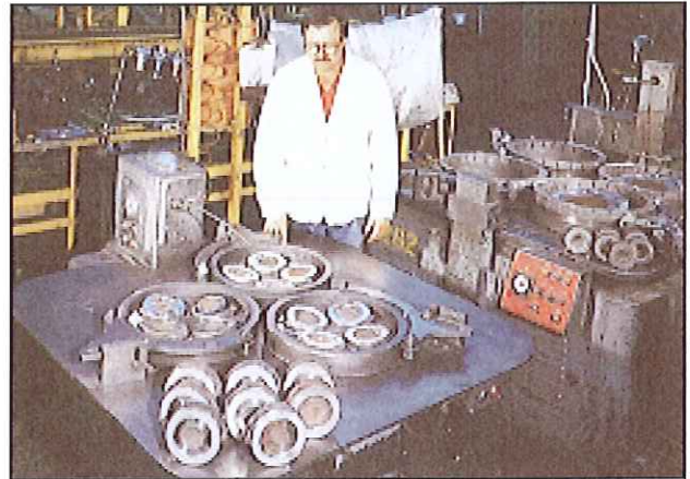
6 Lapping of wedge seating surfaces.
