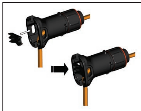
4. Insert banding guide into expediter and snap into place.
