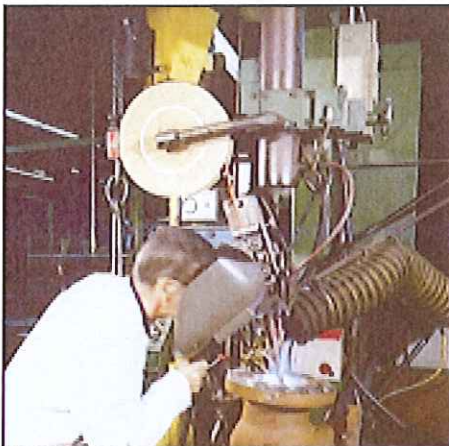
1 Automatic seal welding of Stellite 6 hardfaced seats.
