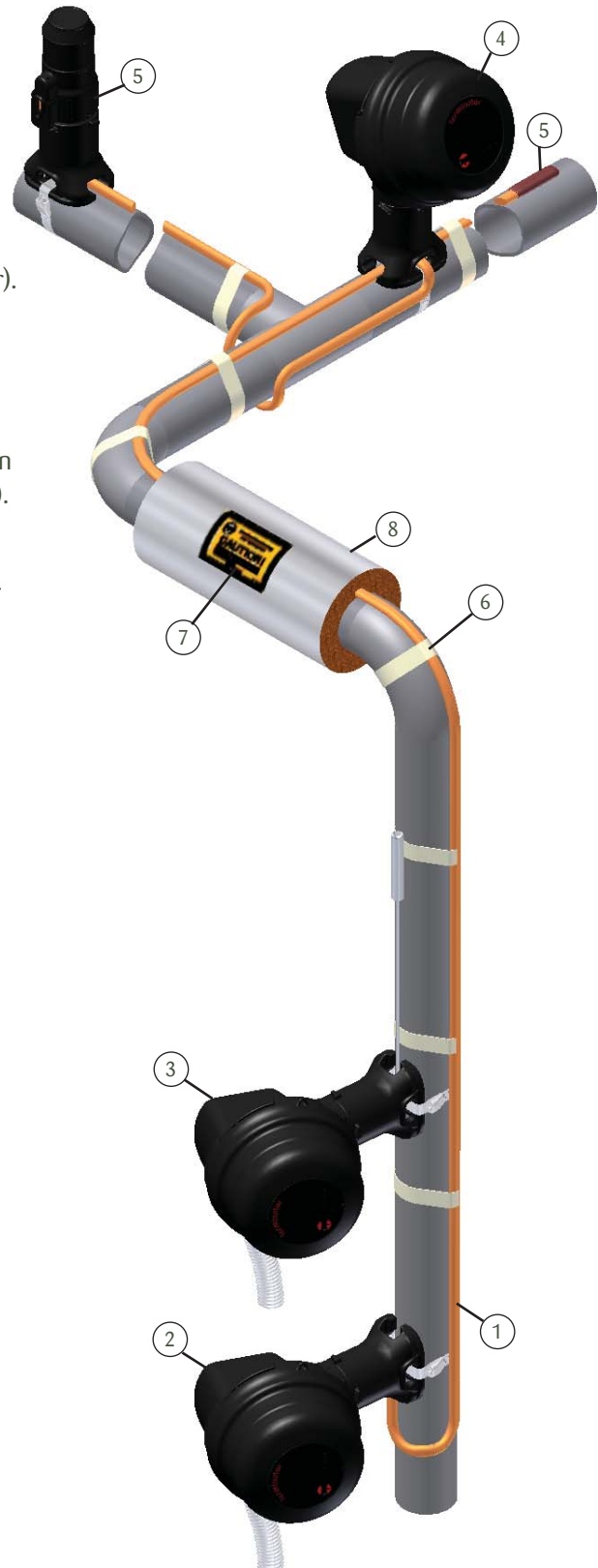
Illustration A: Typical Heat Tracing Installation
