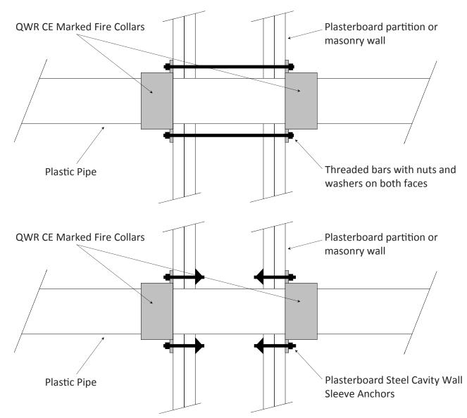
For horizontal pipework one unit should be fitted to each side of the wall.
