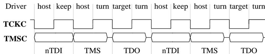
Fig. 4: IEEE 1149.7 T4 two-pin protocol, TAP.7 Advanced Protocol Optimized Scan Format 1 (OScan1)
