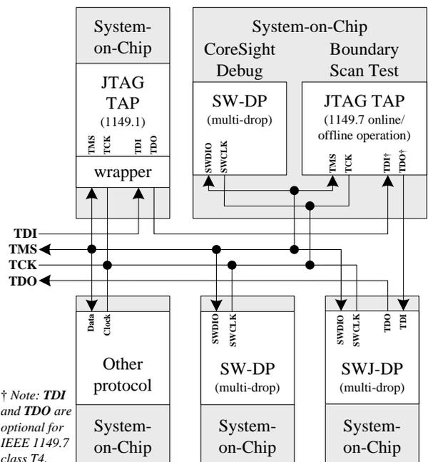
Fig. 9: Multiple JTAG, SW, SWJ (multi-drop) and other protocol devices on a shared connection
