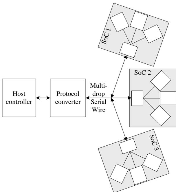
Fig. 8: Multi-drop Serial Wire Debug
