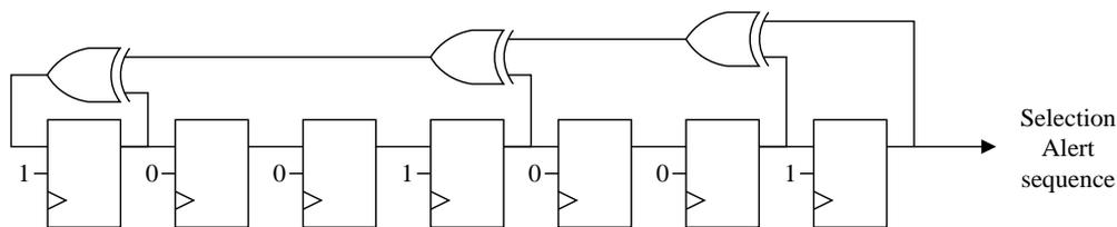
Fig. 10: LFSR for generating Selection Alert sequence
