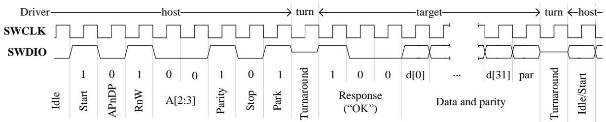
Fig. 6: Serial Wire Debug protocol, read of the ID register
