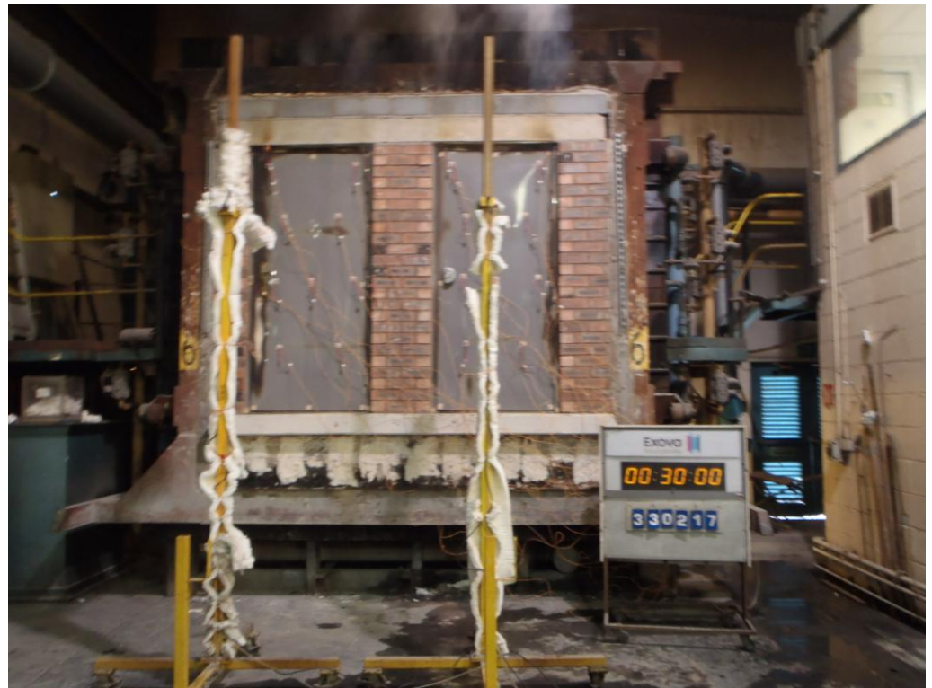
The unexposed face of the doorsets after 30 minutes of testing
