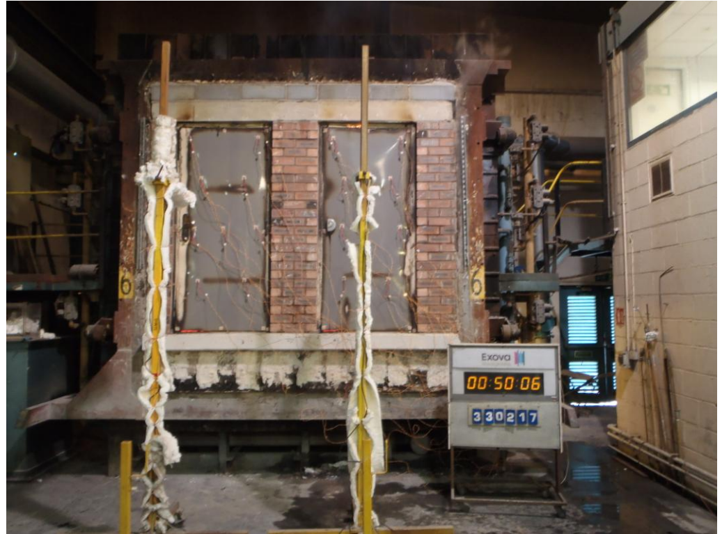
The unexposed face of the doorsets after 50 minutes of testing
