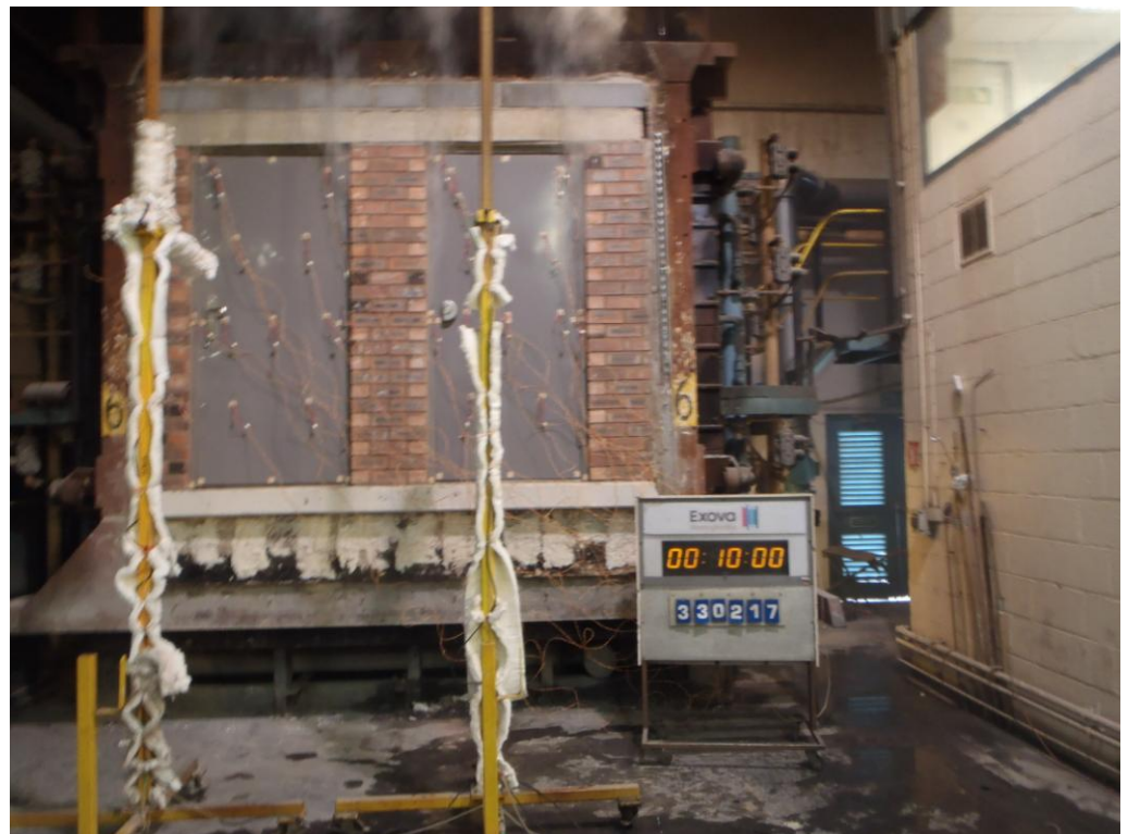
The unexposed face of the doorsets after 10 minutes of testing
