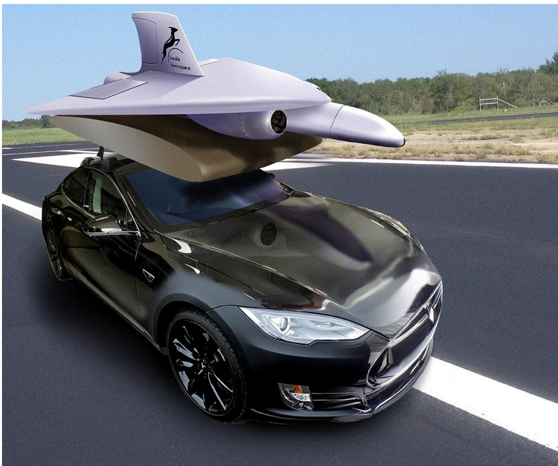
The 1/10 th Scale Swala Vehicle on its launch/capture platform on a Tesla Model S
