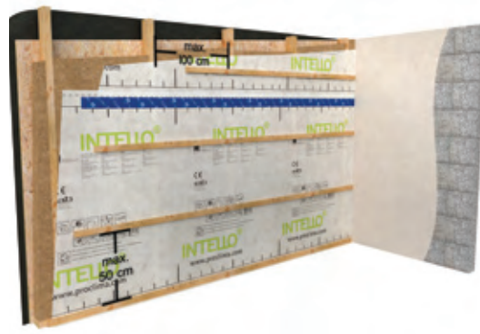
LEFT AND RIGHT: Fully sealed vapour and airtight layers Images: Ecological Building Systems
