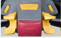
All controls - lift//lower, travel, and horn-accessible from either side of the handle for left- or right-handed operators.
