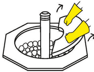
01 Open lid carefully after clearing visible deposits on the top
