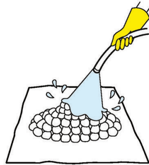
04 In case of heavy sedimentation remove entire gravel from the top module on a tarpaulin and wash it thoroughly with clean water
