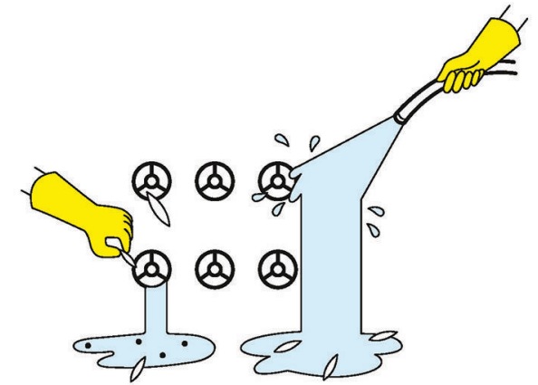
11 Clean all 64 inlets with brush and water, ensure all are clear and clog free
