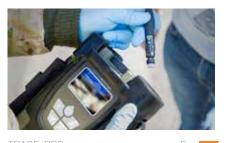
TRACE-PRO Exp IMS TRACE-PRO is a small hand-held, nonradioactive, trace explosive detector utilising IMS technology. It has remarkable integrated evidence collection featuring time/date stamp, complete alarm data, photograph, GPS coordinates and system health. An added benefit is the outstanding clear down time of under five minutes.
