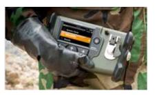
HazMatID Elite CWA • TIC • EXP • NARC FIR This smart, hand-held, solid and liquid chemical identifier utilises Fourier-Transform Infrared Spectroscopy (FT-IR) to detect unknown chemicals, solids or liquids. It performs analysis in one minute or less through its ATR diamond sensor; and has long range, embedded RF wireless transmission suitable for soldiers in the hotzone who need to communicate data to the command post. An optional ClearSampler accessory adds further
